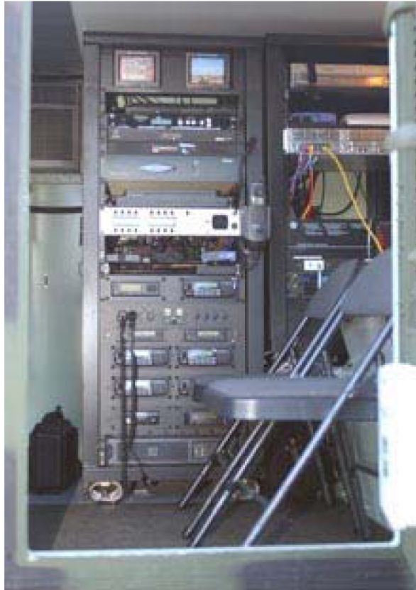
Figure 9. The inside of the IC4U contains just about every emergency communication necessity. Internet link ups, surveillance cameras, CB and HAM radios, etc. This one-man system also features a computer, printer, fax machine, and digital player.
